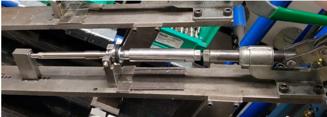
Figure 4. Current snap ring press system.
