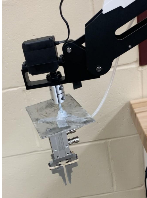
Figure 12. The prototype inner diameter grippers being tested with a robot.
