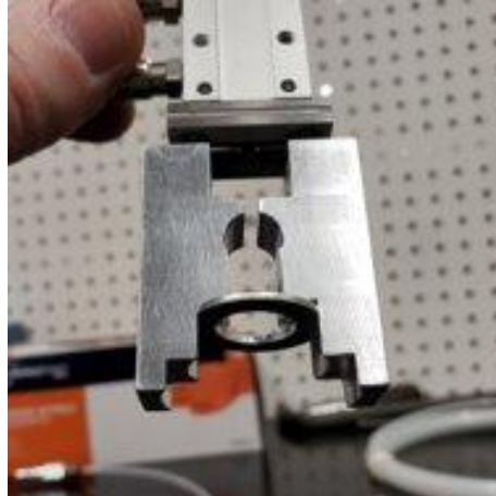
Figure 10. First physical gripper prototype. Could grab each component by the outer diameter.
