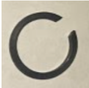
Figure B-8. The snap ring that prevents the washer and teflon from falling off of the disc carrier.
