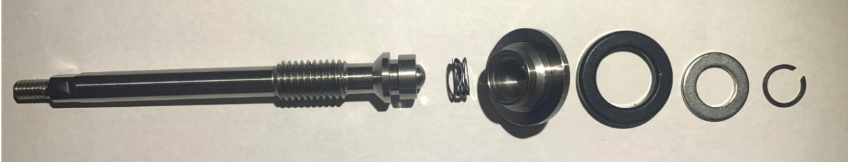
Figure 1. Each component of the hand valve in the order of how they are assembled.
