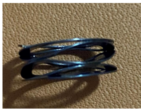
Figure B-2. The wave spring, which goes into the disc carrier before crimping.
