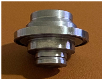
Figure 5. Side view of the disc carrier to see the snap ring groove. The groove is the small indented section at the bottom of the disc carrier.
