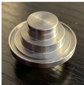
Figure B-4. The bottom of the disc carrier, where the teflon, washer, snap ring, and mandrel attach.
